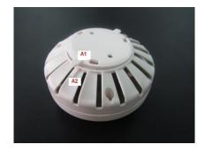
Lock in position by giving a clockwise quarter turn. This clockwise turn turns on the sealed-in battery. i.e. the power on the device is turned on as soon as it is in the locked position.
