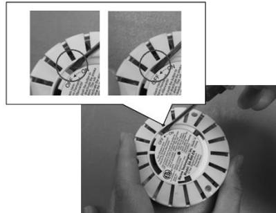
**Use a screw driver to push the button to “Off” position in order to deactivate the smoke alarm. This will deactivate the alarm, stop the low battery “chirp” and render the alarm safe for disposal by draining the battery.**
